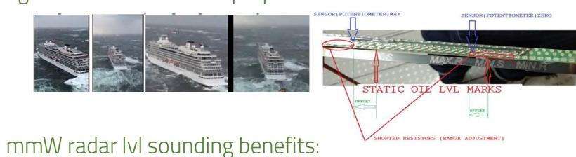
increased accuracy, fast acquisition compared to manual sounding presently used, in case of vessel grounding time gained to abandon vessel decision improve survival chances.
