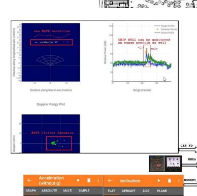
Radar measures wave waterline shape and wave clutter dynamics
